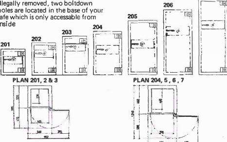
EXTERNAL HEIGHT 602 (1'11%") 752 (2'5%") EXTERNAL WIDTH 560 (1'10'4") 560 11'10 11 EXTERNAL DEPTH ,520 (1'8%") 520 (1'84") INTERNAL HEIGHT 447 11'5%"] 597 (1'118") INTERNAL WIDTH 405 (1'3 %") 405 (1'3 4") INTERNAL DEPTH 330 (1'1") 330 (1'1") CUBIC CAPACITY **TOTAL WEIGHT** 365kg (805lb) 415kg (915lb) 445kg (981lb) 655kg (1444lb) 790kg (1742lb) 925kg (2039lb) 1040kg (2293lb)
