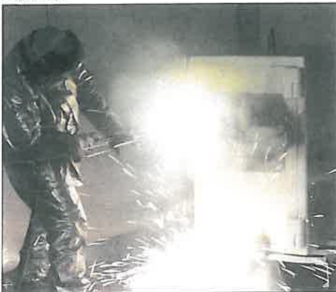
UL Test Engineer Attacking Door Jamb with Torch.
